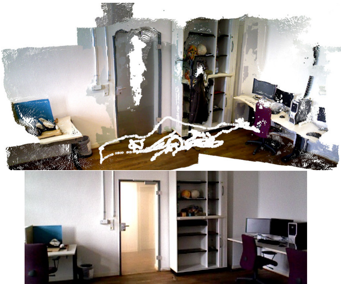
Figure 1.1: Top : Scene view reconstructed in our program. Multiple dense textured depth maps from different view points form a consistent scene model. The white curve along the bottom displays the live camera trajectory. Bottom : The same scene in the real world (not recorded at the same time, hence the differences in lighting and the missing hat stand in the bottom image).
